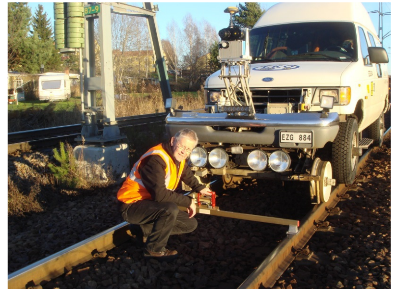
Lars Lundberg checking the track cross-level as part of the accuracy test
